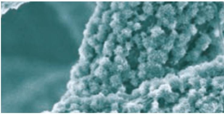
**Fig 6** Highly reactive calcium phosphate nano particles are integrated into biodegradable PLGA by electrospinning. The formed fibers allow fast mineralization due to the reactive nano particles.
